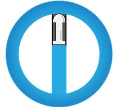
The CRUSH GAUGE is on the rotational edge of the Resin insert and will show the mismatch of alignment holes occurring due to worn square drive surfaces and socket.
